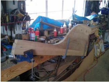
Rudder constructed with the bronze castings patterns fitted in preparation for the real thing.
