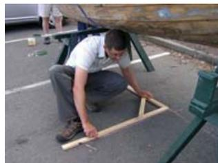
Dougal sets out a grid by which to take the laser measurements
