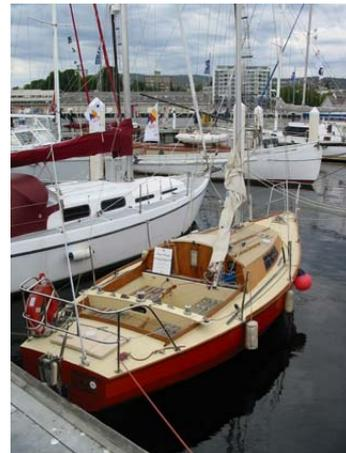
Rob Wallis's "Westwind" a 24' Marine Plywood Clinker, mast head sloop.
