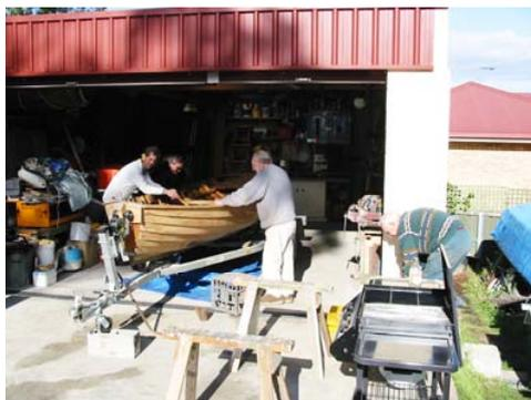
*Fixing roves and rivetts*
